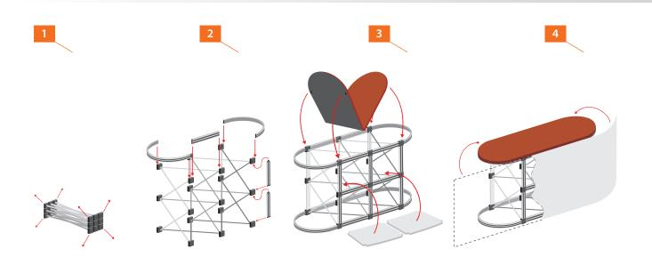
Remove pop up frame from carry bag. Erect top locating studs are upper most.
