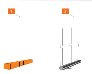
Remove your roll up and bungee pole from the carry bag. Take the poles and allow all three sections to slide together. Insert the pole into the casette, ensuring that it is fully located.
